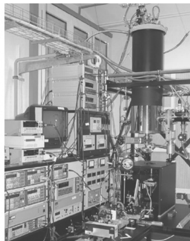
Fig. 7. Operating principle of a cryogenic electrical substitution radiometer (left) and the PTB radiation thermometry cryogenic radiometer (right).
