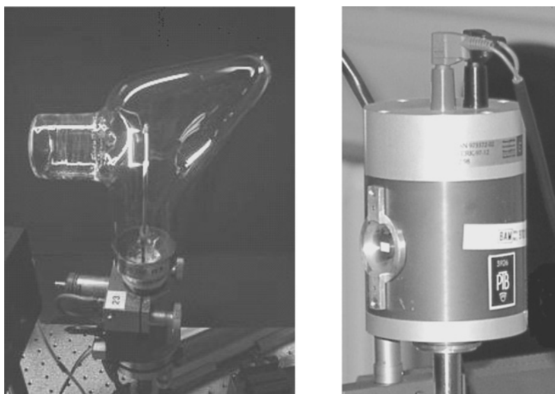
Fig. 9. Spectral radiance transfer standards: a tungsten ribbon filament lamp (OSRAM Wi17/G) operated at radiance temperatures ( \lambda = 650 nm) from 2300–2500 K (left) and an integrating sphere type, low-intensity spectral radiance standard (Gigahertz BN9701) (right).
